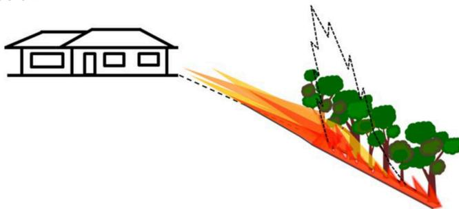
Schematic diagram of a fire burning up a positive slope towards a house. The orange and yellow flames represent the case of eruptive fire spread, in which the flames have attached to the surface. The black outlined flames represent the case of a separated plume, which is the situation depicted in AS 3959.<sup>vi</sup>
