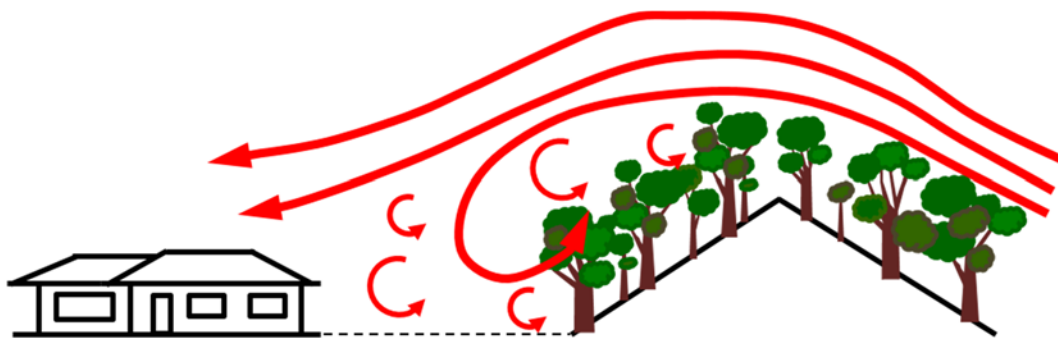
Figure 7: A situation that would be assessed as an 'upslope' effective slope in AS 3959. However, in this situation the winds (red arrows) over the 'upslope' effective slope have separated from the surface and have formed a lee eddy.
